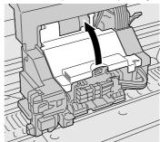
8 Pull the printhead lock lever completely forward to open it.
